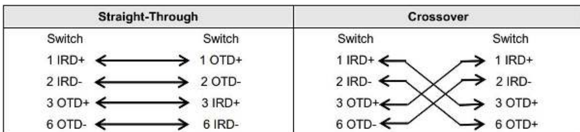
Figure A-2 100BASE-TX/10BASE-T Connection
